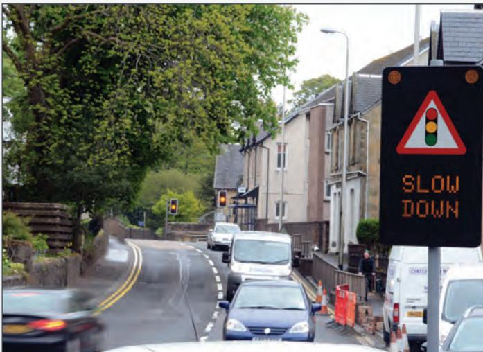
The vehicle speed is wirelessly relayed to the traffic signals and if speeds are recognised as being above 30mph then the signals are programmed to turn to red, thus stopping the speeding traffic and increasing overall journey time through the village.
