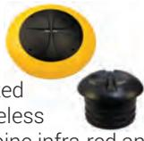
The M301 surface mounted and M302 embedded wireless occupancy sensors combine infra-red and magnetometer detection technology, using a sophisticated algorithm to ensure detection is highly accurate and reliable under all conditions, and is equipped with a low power secure radio transmitter.
