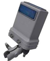
All repeater units are battery powered and require no external power supply or cabling. There are two variants of M115 Repeater; the solar powered variant has a battery life over 10 years and is non-replaceable whilst the battery variant has a replaceable lithium thionyl chloride battery offering a seven year life.
