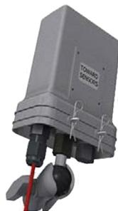
The access point uses a wired connection to relay the sensor detection data via a:
