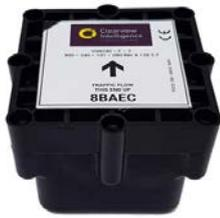
The M100 uses 3-axis magnetic field sensing, with each sensor providing a detection zone of 2m in length by 1.3m width. Sensors must be deployed within 35m of an access point or repeater and communicates vehicle presence within 125 milliseconds allowing for real-time operation.
