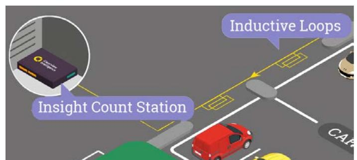
software (Insight Parking). Data can be used for real-time and historical analysis or fed through to VMS and mobile phone applications to aid parking guidance.
