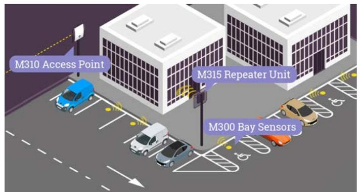
The wireless network can be extended using battery powered repeaters providing further coverage across a car park. The parking bay sensors are available as an in-ground embedded stud fitted flush to the road surface or surface mounted.
